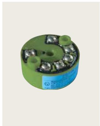
A transmitter can be assembled inside the connection head to convert the electrical values generated by the sensor into an analogue (4/20 mA) or digital signal output. Transmitters are available with a fixed, selectable or programmable range (Smart) with HART™, PROFIBUS™ or FIELDBUS™ protocols.
